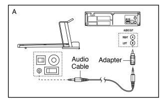
B. Plug one end of the audio cable into the jack on the front of the treadmill near the power cord. Plug the other end of the cable into the included adapter. Plug the adapter into an RCA Y-adapter (available at electronics stores). Next, remove the wire that is currently plugged into the AUDIO OUT jack on your VCR and plug the wire into the unused side of the RCA Y-adapter. Plug the RCA Y-adapter into the AUDIO OUT jack on your VCR.
